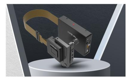
The HDSLM80R Pro Liquid Crystal Spatial Light Modulator consists of a driver, FPC flexible cable, and LCoS temperature controller. Configured with the TEC controller and LETO TEC CONTROLLER software, it is used to set the operating temperature of the LCoS optical chip based on the ambient requirement.
